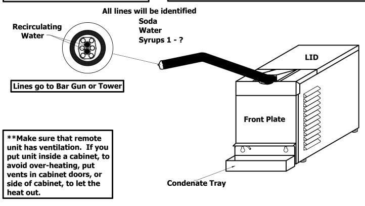
The incoming water, syrup, CO2 gas, and electric lines all come out of the unit behind the "Front Plate" in the center. It is best to bring the lines straight back, under the unit to keep them from kinking. You can raise the glides to keep from kinking the lines \*\*\*Connect all lines and turn on the water supply, BEFORE turning the power switch to the "ON" position.
