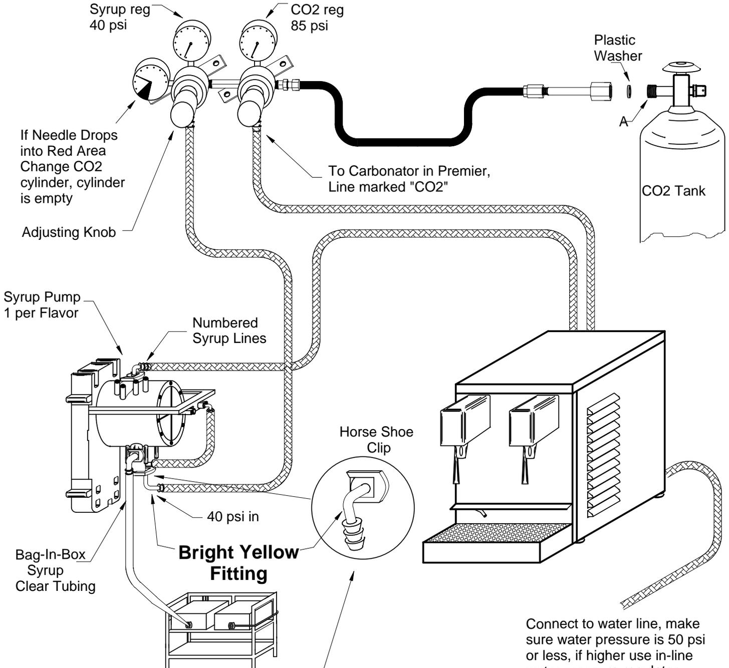
Connect to water line, make sure water pressure is 50 psi or less, if higher use in-line water pressure regulator
