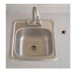
Drill a 1 3/4 inch hole in the countertop. If you can only drill a 1 1/2 inch hole, it is possible to make it fit, however you will need to taper the edges of the hole to allow the top of the Pop-up assembly "sink" into the countertop. Remove either the Jamnut or top ring to install in a counter. In cases where the counter is too thin to tighten Jam-nut, a length of 1 1/2 inch PVC pipe can be cut and used as a spacer.
