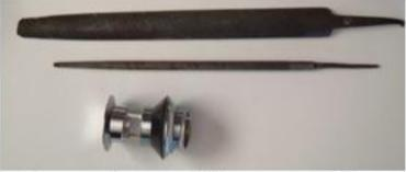
Use a round or curved file to remove all burrs from cutting, leaving the inside edges smooth.
