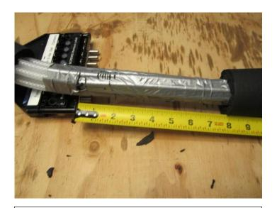
Shove the insulation back pulling on tubing. Try to get 8" – 10" away. Further away makes it easier to connect to the bar gun.
