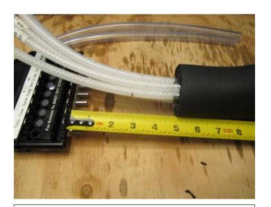
Pull up the insulation back over the U bend at least 4" past where the U bend is located.
