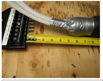
Tightly duct tape the insulation to the rest of the lines to keep the air out. If this is not done correctly the duct line will pull in moisture and cause the duct line to sweat. **VERY IMPORTANT!**
