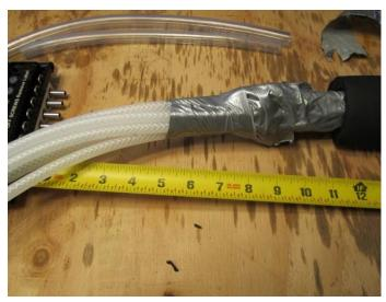
Tightly duct tape the U bend to keep the air out all the way up to within 5"- 9" of where the manifold is located.
