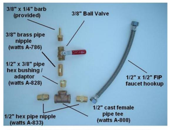
Remember: Wrap all brass to brass threads with Teflon tape, and tighten all fittings with a wrench, pipe wrench or pliers to avoid any leaks.
