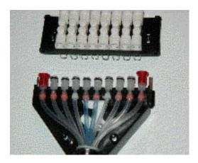
Use the "White" button to slide the the manifold apart.
