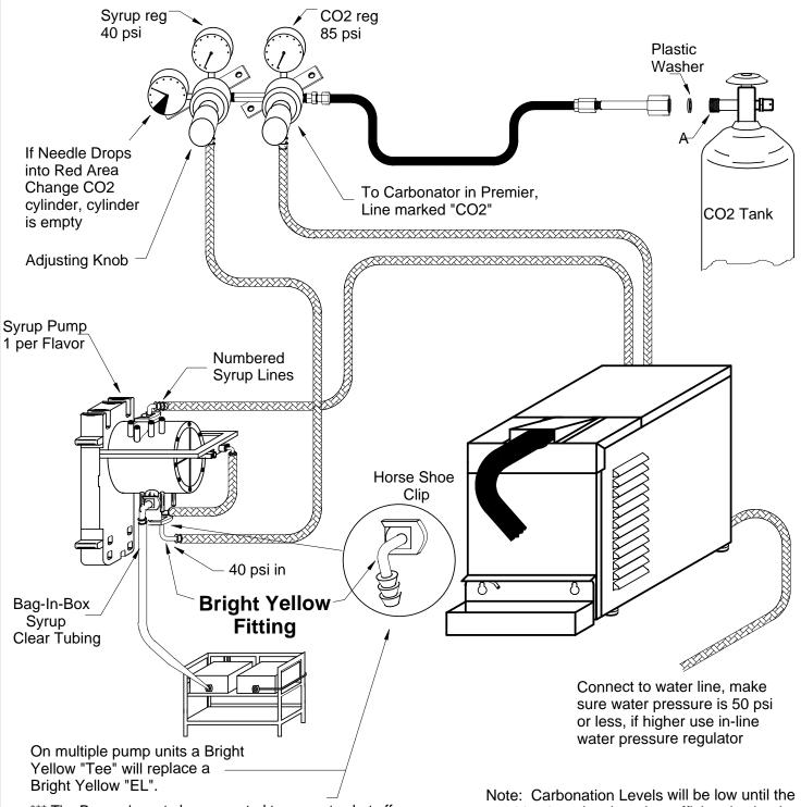
\*\*\* The Pumps have to be connected to syrup, to shut off, or they will keep pumping... You can disable the pump, by sliding the "horseshoe" Clip toward you, and pull the CO2 fitting out, Stright down, and it has a "auto-shut" off built into it.
